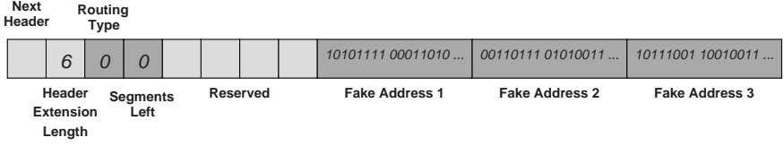
Fig. 9. \beta Covert Channel in the Routing Extension Header , when Alice creates fake addresses in a packet that did not originally a routing extension header
